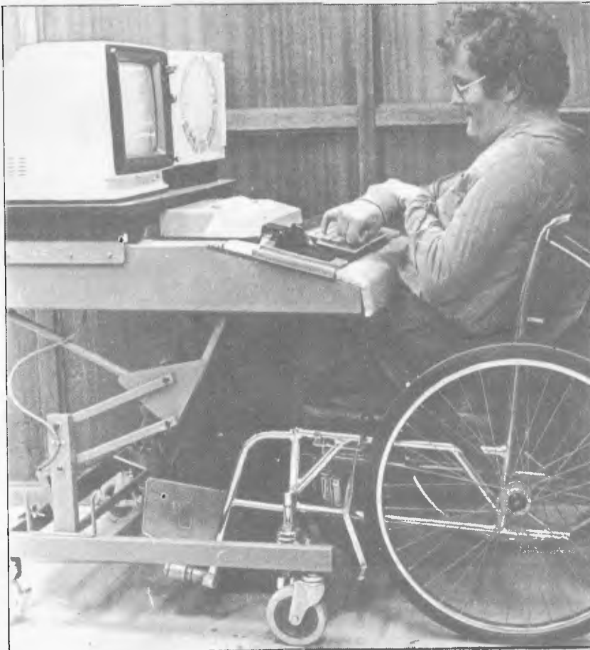
Leigh Lockrey operates an Apple II micro SCAT (Scanner Apple Touch Keyboard) system mounted on a trolley to provide a fully mobile base.
